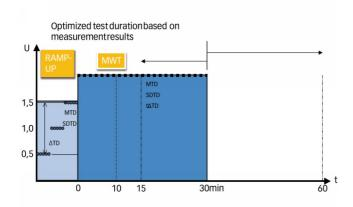
More information in less time: The cable condition is determined before the actual MWT - cable testing and dissipation factor measurement are combined. The subsequent MWT often takes less time than a normal cable test.
