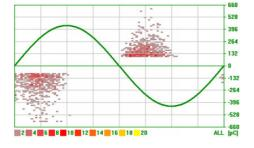
Partial discharges in the insulation, such as electrical trees, primarily occur close to the zero crossing (see image), external partial discharges typically become more frequent at the maximum of the sinusoid. With the help of the optional phase-resolving from BAUR Pruef- und Messtechnik, this becomes more visible and users can limit the type of cable fault better.
